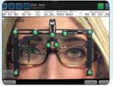
centration allows eyewear measurements to increase an optician's measuring exactness in a number of ways. These "as-worn" measurements take monocular PDs more accurately by taking into account how the frame sits on the customer's face. This is in contrast with the pupilometer, which captures PDs anatomically and does not take into account frame fit and nosepad adjustments.
