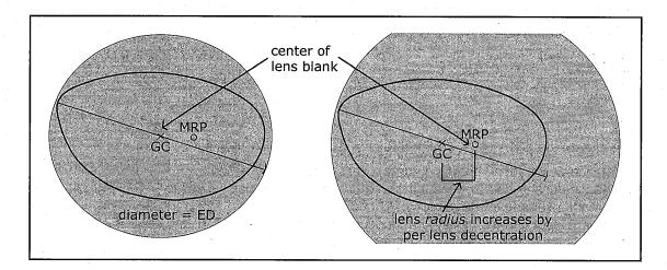
If there is no decentration of the optical center, the minimum blank size is equal to the ED of the frame. This occurs in the following situations:
